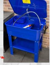
2 Correct Cleaning Fluid. TQB Brands recommends the use of our Tradequip 5082T & 5083T biodegradable aqueous parts washer cleaning fluid to be used at a dilution rate of five to one for best cleaning results and parts washer pump longevity.
