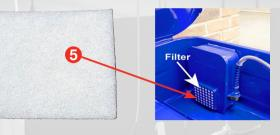
Regular maintenance is essential for best results. Cleaning fluid should be changed regularly where sludge build up will settle in the bottom of the tank. This will reduce the effective cleaning ability of the parts washer and should be changed monthly or more regularly if frequency of use is higher.
